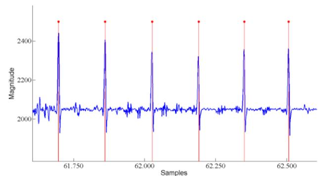
**Figure 3** ECG signal from the FitnessSHIRT (blue) and the results of the R-peak detection (red)
